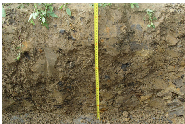
Fig. 1 Photographs of the 0.55 m vertical lignitic mine soil profile, about 0.9 m in width
